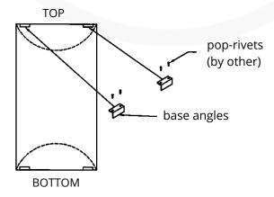
2 Attach the two 4" long base angles (with pile velcro & PSA hook) to the bottom of the diffuser from the Gel -coated sid. Insert the white headed pop-rivets (by other) thru the pre-drilled holes in the base angles and the diffuser.
